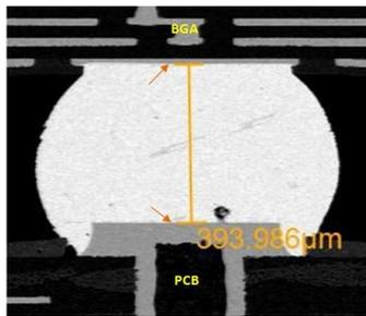
Figure 2. Standoff measurement
